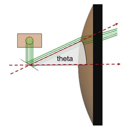
Laser scanning systems, with the help of e.g. a galvanometer, is capable of deflecting laser beams into predefined directions. And, in combination with focusing optics, such systems are often used for precise laser material processing. A scanning system consisting a dualaxis galvanometer and an aspherial focusing lens is modeled in VirtualLab. The rotation of the mirrors are modeled as in the practical case, and the focused laser spot at different scanning angles are examined.
